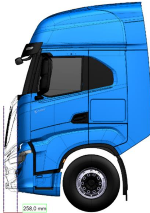
Figure 16: New cabin concept with aerodynamic front-end.
