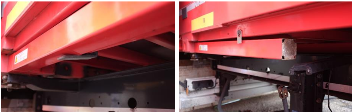
Figure 24: The supporting legs position of the swap body during driving conditions.
