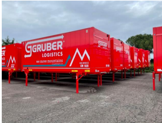
Figure 23: The supporting legs of the swap body.
